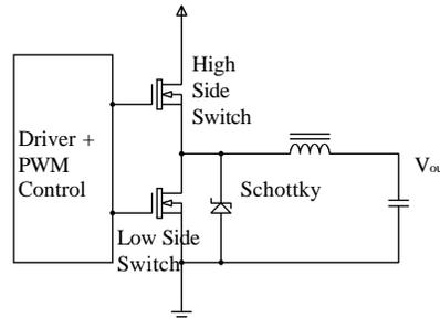
Figure 1. Typical POL synchronous buck schematic.
