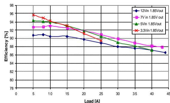
Figure 17. Efficiency of the Si4770CY at 500kHz
