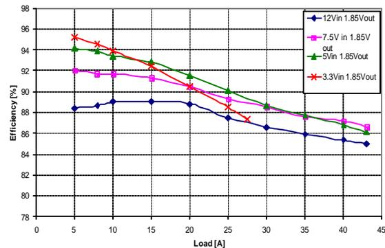
Figure 16. Efficiency of the Si4770CY at 750kHz
