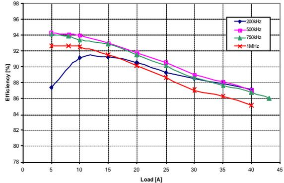
Figure 13. Efficiency of the Si4770CY with 5 Vin, 1.85 Vout.
