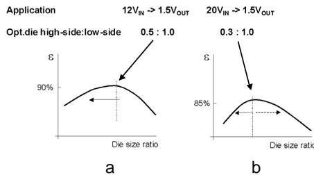
Figure 2. Effect of die ratio on efficiency.
