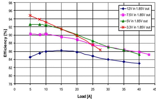
Figure 15. Efficiency of the Si4770CY at 1MHz
