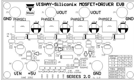
Figure 9. Four-phase evaluation board, implementing SO-16 packages.
