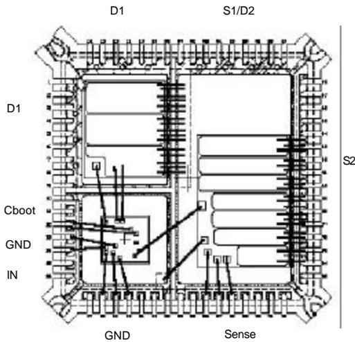
Figure 10. Schematic of new MLF package.
