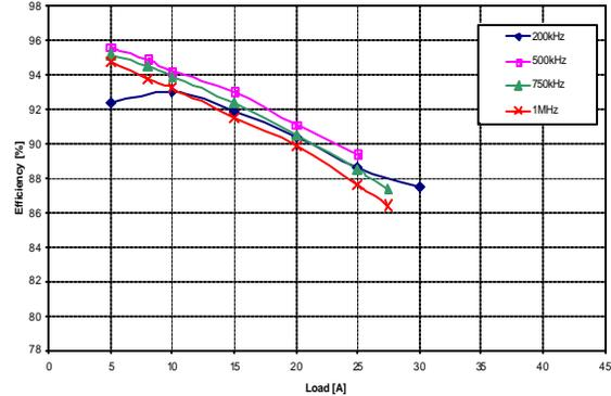
Figure 12. Efficiency of the Si4770CY with 12 Vin, 1.85 Vout.
