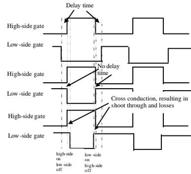
Figure 3. Timing of the high-side and low-side gate signals illustrating cross conduction
