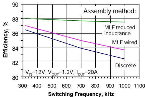
Figure 11. Simulations showing improvement in efficiency with packages.
