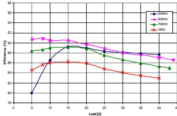
Figure 14. Efficiency of the Si4770CY with 12 Vin, 1.85 Vout.
