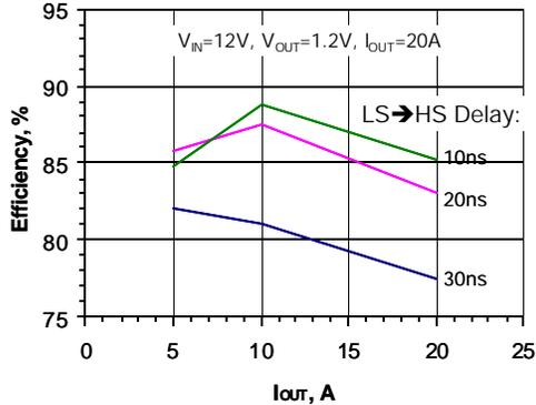
**Figure 5. Simulation showing the improvement in efficiency with the reduction of dead time.**
