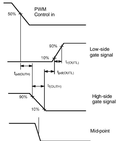
Figure 4. Adaptive high-side turn-off low-side turn-on control.
